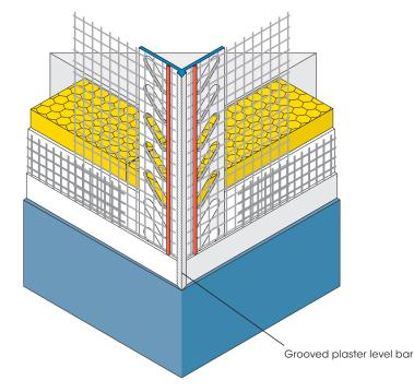
The APU Corner Bracket with fabric TOP-TEX is suitable for thin and fine layer plasters.
