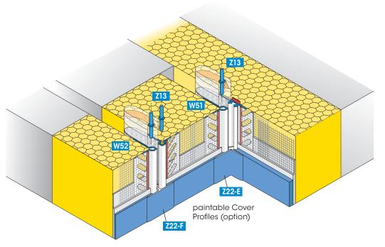
The Expansion Joint Profile consists of two plastic profiles with plaster level bars and a Sealing Joint Loop made from flexible fiber-reinforced plastic foil. Both sides are equipped with fabric parts approved for ETIC systems, UV welded onto the profile.
