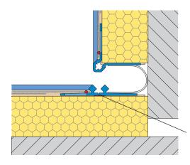
Flat profile can be used by bending in a right angle also like W52 for applications on even surfaces.
