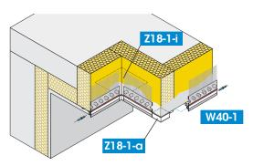
Corner Element Z18-1 in this case at Border Profile DROP-TEX-UNO W40-1
