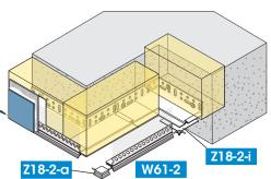
the Corner Element can be trimmed with Shears (Z12) to fit as required.
