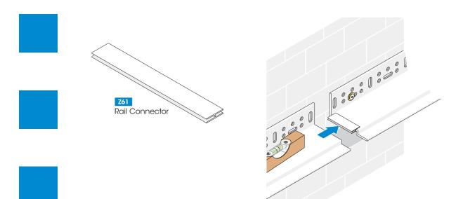
The Rail Connector Z61 simplifies flush aligned displacement-free aligning of base/mounting rails with material thickness up to 2.5 mm. For this, portions of the bars are cut with Trimming Shears Z12 as required.
