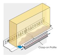
The Clasp-on Profiles are slid in below the insulation board onto the stepped bending and aligned in a flush direction into the fixing mortar with Plug Connectors Z13 between two profiles. The Clasp-on profiles should alsways be installed overlapping the Base Rail joints for stabilization.
