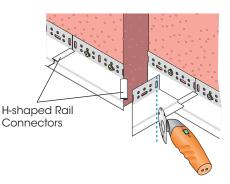
Cut the corner parts of Base Rails in place using Shears Z10 or a Multimaster tool (type FEIN).
