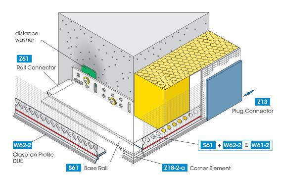
The Base Rails are made of plastic with a stepped bending for taking up its counterpart Clasp-on Profile with fabric 12.5 cm and Drip Edge. It is suitable for insulation thicknesses of 50-200 mm in thermal insulation composite systems with rigid foam/mineral fiber boards and fabric filler of 4–8 mm. For improved adhesion of the plasters the transition to the Drip Edge is grooved.
