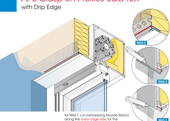
Plaster borders in thermal insulation composite systems also require a secure solution with regard to water-guiding and drainage downwards.
